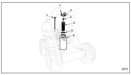
Figure 4-13 Hydraulic Oil Filter Assembly
